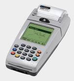
NURIT 8000S provides a 2/14" by 2 1/4" (128 x 128 pixels) backlit graphical display, with touch screen to support electronic signature capture.
