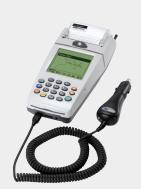
The NURIT 8000S vehicle adaptor enables rapid charging of the device's battery using the vehicle's 12V or 24V electrical power socket.
